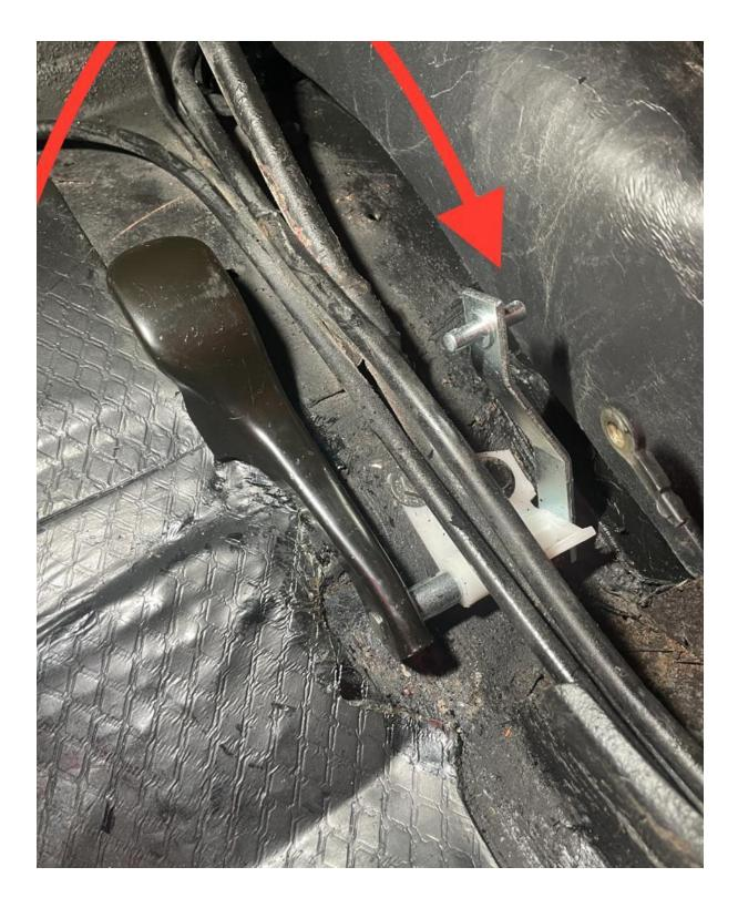
The little bracket attached to the cable needs to be bolted in the body somewhere along where the red arrow is pointing. You will see a little bolt there when you remove the old cable.
