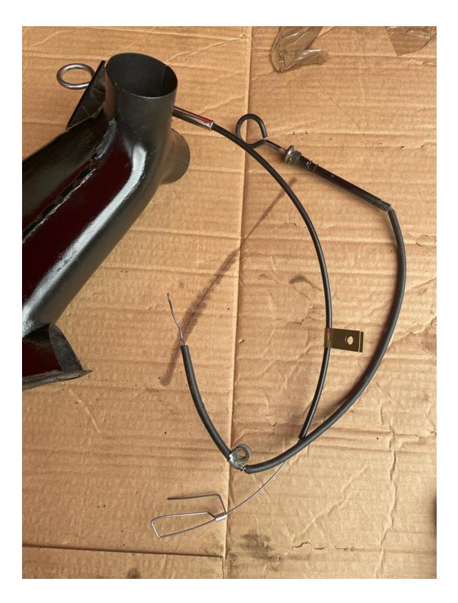
The end of the hand throttle goes where the arrow is pointing you need a fat washer with a little pin to hold it in place. The cable when you pull it goes in & out accelerate or decelerate it works like a cruise control.
